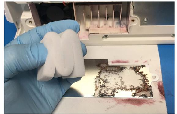
12. Press the new ink filter into the ribs as shown.
