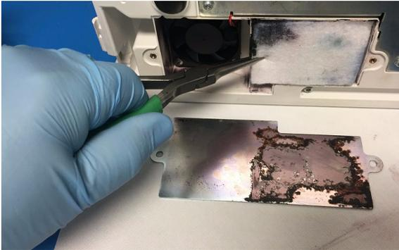
9. The ink filter will be saturated with ink making it messy to handle. Use a pair of needle nose pliers to remove the filter and discard it.
