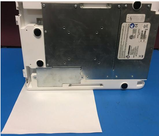
5. Use a T10 screwdriver to remove the two screws securing the fan cover. Save the screws for step 14.
