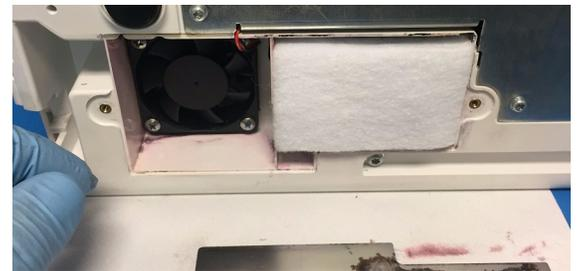
14. Place the fan cover into position and secure with the two screws from step 5 using a T10 screwdriver.
