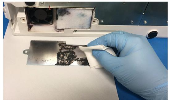
8. The ink pad will be saturated with ink making it messy to handle. Use a pair of needle nose pliers to remove the pad and discard it.
