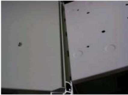
10. Make sure that the shelf is still level right-to-left with the SLS 500i on it. If necessary, remove the drawer and use the three set screws on the shelf rail to readjust the level of the shelf. (IMAGE FROM PREV. GUIDE) (NEW PICTURE?)
