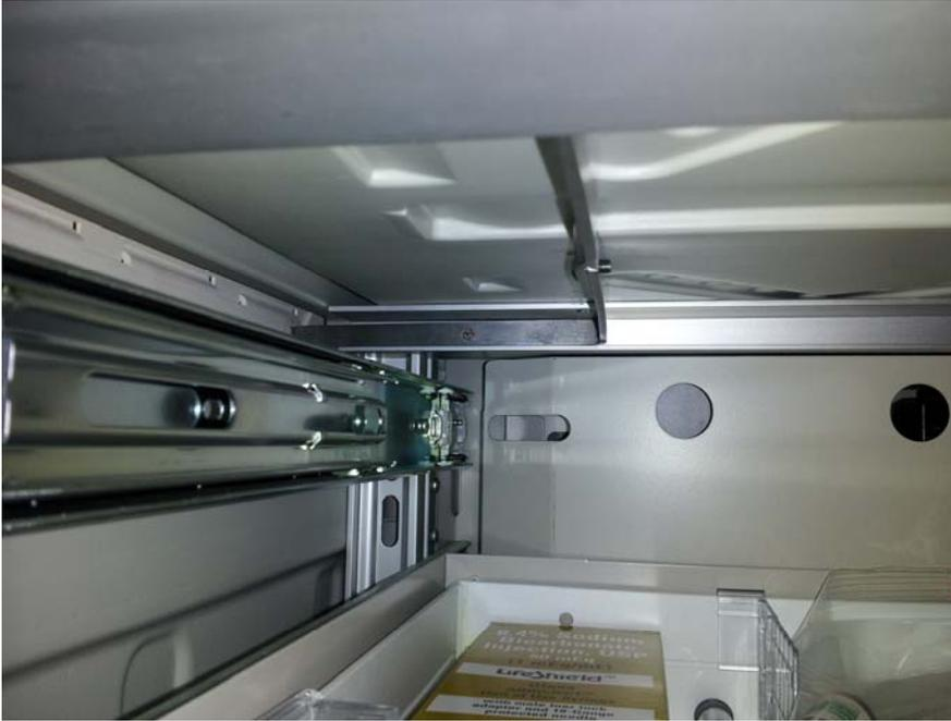
5. Install the lower brace into place as shown with two supplied 6-32 Philips head screws.
