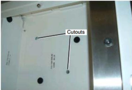
A close up of one of the SLS 500i threaded holes as seen through the cutout in the shelf frame is shown in the following figure.
