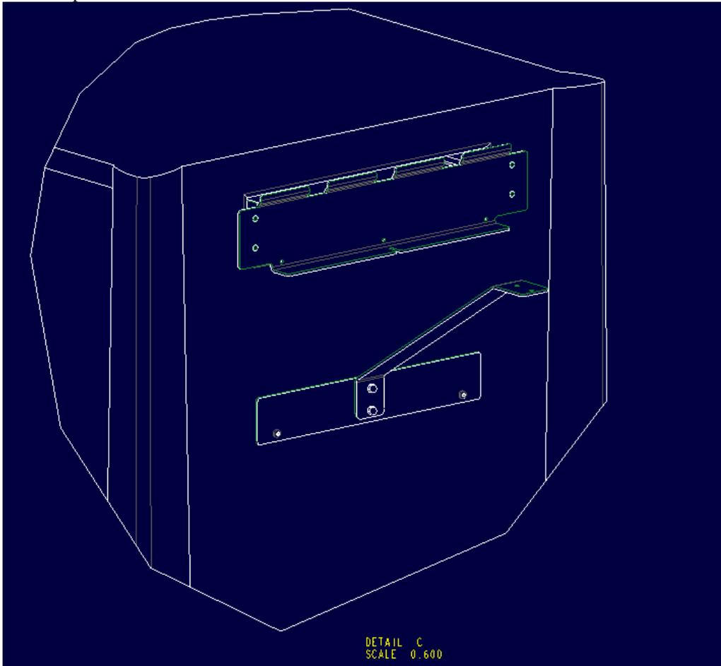
7. Remove the acorn nut from the bottom of the shelf that is closest to the side where the shelf frame mounts to the shelf rail, as shown in the following figure. (IMAGE FROM PREV. GUIDE)
