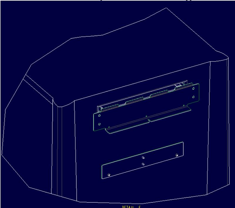
6. Place the Support Bracket on the Lower Brace as shown and secure in place with the two acorn nuts provided.
