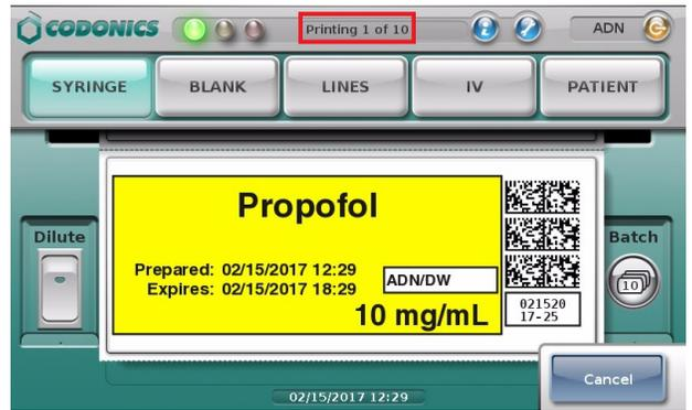
10. When the batch is completed, if Strip had been selected on the Batch Mode Configuration screen, a dialog box will be displayed summarizing the job and asking if you would like to cut the strip. Select OK. SLS PCS will automatically cut the liner.
