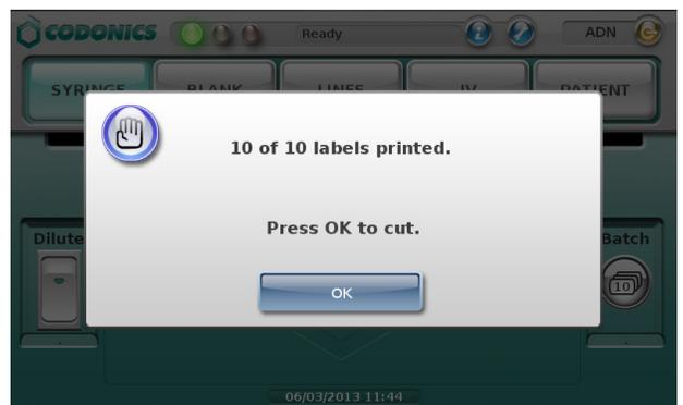
**WARNING:** Do not pull the strip of labels or try to tear the strip of labels. This can cause jamming and/or damage to the SLS PCS.
